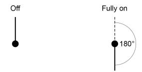
When fully on, water flows out of the tap at 14 litres per minute.
